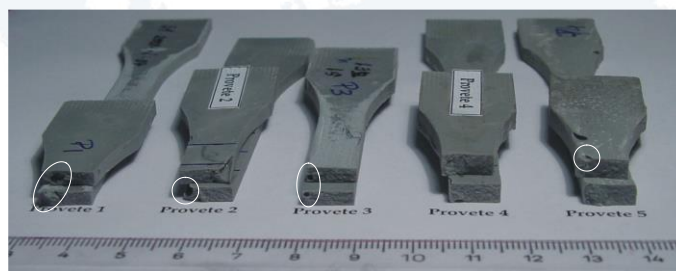
Figure 9. Voids on the fracture surfaces of the epoxy adhesive specimens.
